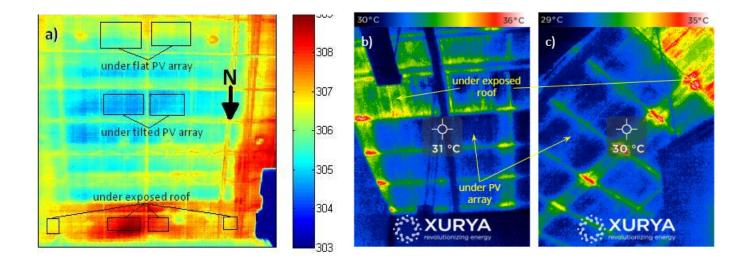
Thermal infrared image of the ceiling shows cooler area below the PV array compared to areas with normal roof: (a) From a result of scientific study (<u>https://phys.org/news/2011-07-solar-panels-cool.html</u> (b) From Xurya's site in Indonesia. Solar panels have the ability to **block sunlight from heating the roof**. This results in:
